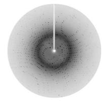
**Fig.2:** Diffraction frame recorded on an elastase crystal. Scan width 1° (Omega), exposure time 300 sec. Crystal-Detector distance 150mm. Resolution at edge (170mm from center): 1.89 Å
