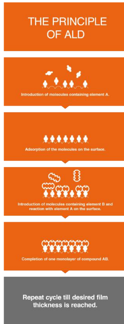
Figure 2: The principle of ALD film formation (image credit Picosun)
