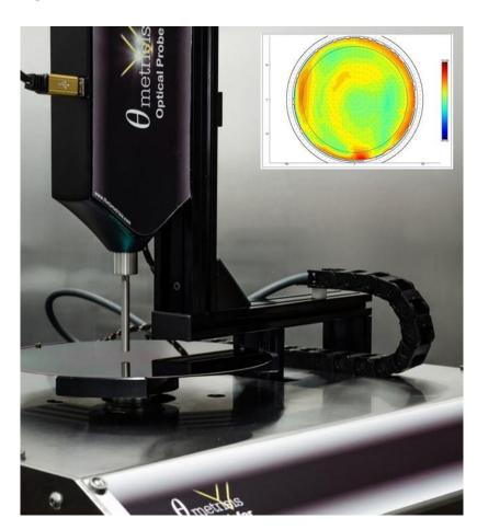
The unique optical head accommodates all optical parts: the spectrometer, the hybrid light source (lifetime, 20000h), the rigid reflection probe. Therefore, excellent performance in terms of accuracy, reproducibility and long-term stability is guaranteed.
