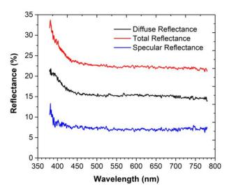
Total, Diffuse and Specular Reflectance measurements of a painted aluminum sample, as they were measured using an FR-pRo tool equipped with an integrating sphere
