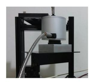
FR-IntSphere kit along with a FR-pRo tool consist of a full solution for reflectance measurements, without any need of additional components. The integrating sphere is compact, easy to operate, made of a highly reflective, Lambertian surface (PTFE), with a sample port diameter of 10mm.
