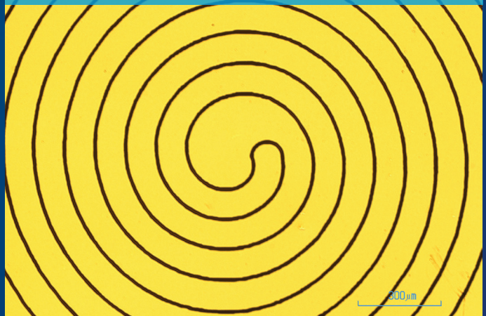
Curved and very long 10 μm microchannels
