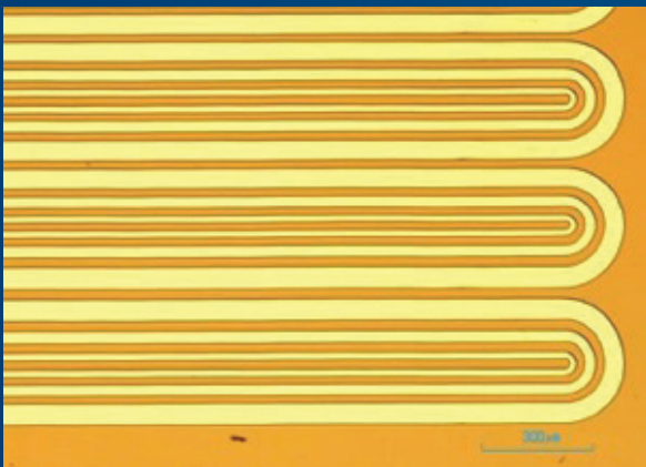
Curved and very long 10 μm microchannels
