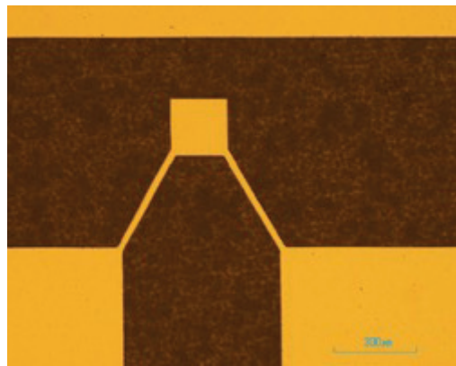
MEMS oscillator photomask
